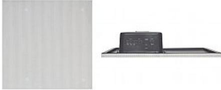
The Tavor 8-T High Performance Powered Ceiling Tile Speaker features a 40 watt built-in class D power amplifier, three inputs, Kevlar(R) woofer, four pivoting titanium tweeters, complete K-coverage ESD™ (Equal Sound Dispersion) design for almost 180 degrees of sound dispersion, magnet held grill (with two security screws) for time saving installation, and a 2nd-level cross-over
